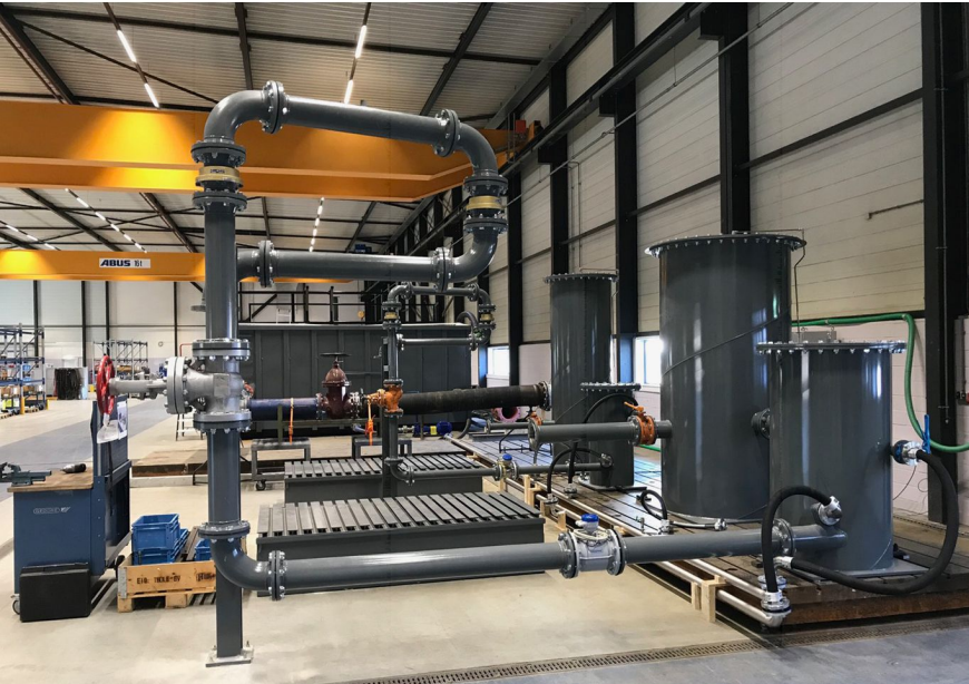
Closed test loop 80-150 OH type of pumps (API)
