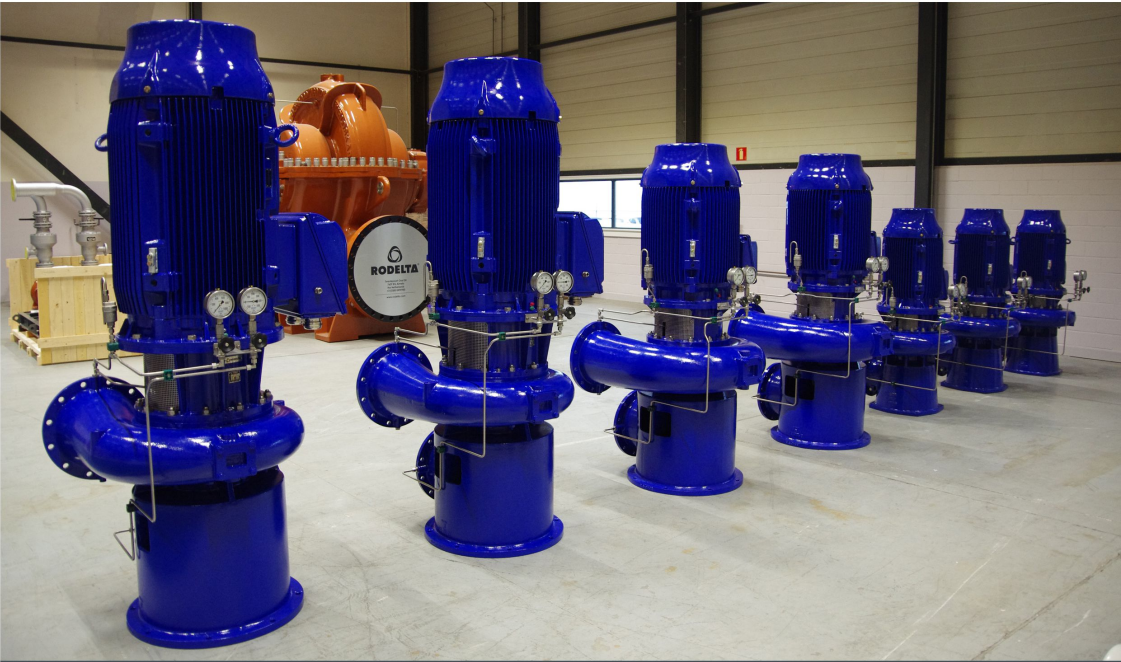
Press and suction pipe are adjustable for different connection possibilities
